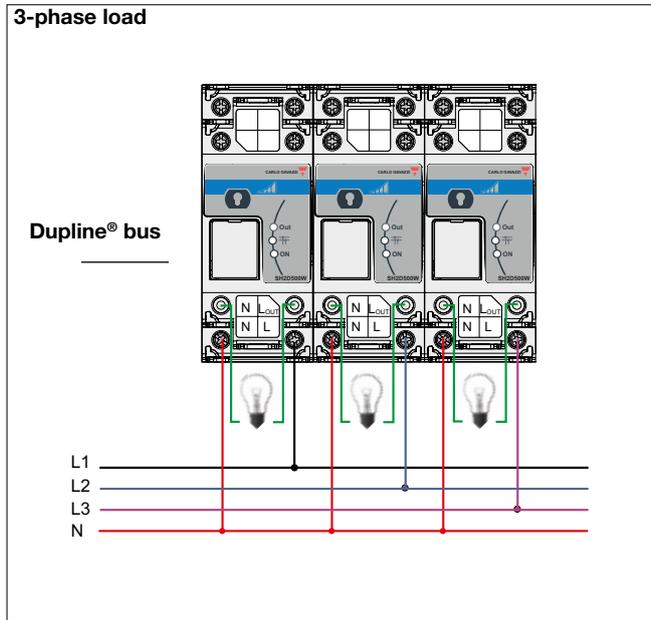
Note: The distance between the dimmer module and the light should not exceed 25 metres
