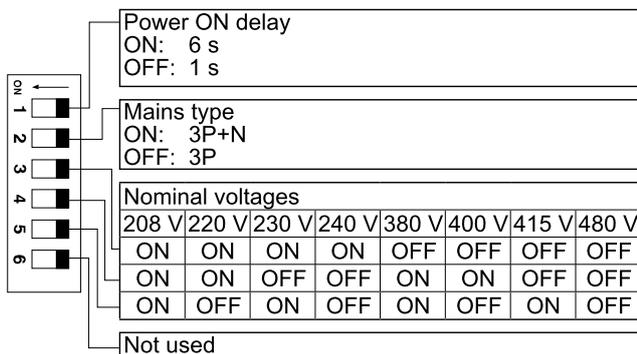
**Fig. 1** DIP switch settings table M44
