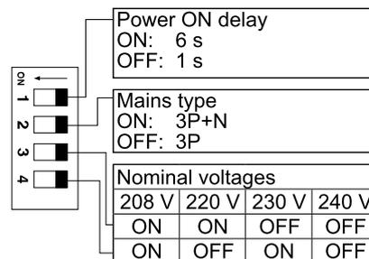
**Fig. 2** DIP switch settings table M23
