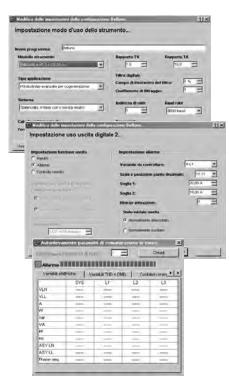
The EM2426Soft allows to create in an easy way the requested configuration of the instruments with the relevant system setting (CT and VT ratio, system, alarms, etc.), it is able also to manage an archive of configurations which may be easily recalled. A pre-set programming configuration can be downloaded and if necessary modified.
