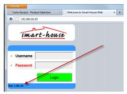
Start your browser, enter the IP address of your controller, and check the release number in the bottom of the information box. (Indicated in the figure left with the red arrow).
