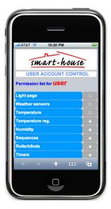
Scrolling down the list of the Function pages, you will find the setup access for the rooms: if only the checkbox "View" is selected, the user will only be able to see lights, temperatures, alarm status,..., but not to control them. In this case the symbol will be shown on the red side of the function.
