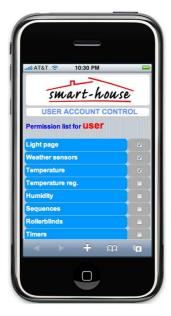
Scrolling down the list of the Function pages, you will find the setup access for the rooms: if only the checkbox "View" is selected, the user will only be able to see lights, temperatures, alarm status,..., but not to control them. In this case the symbol will be shown on the red side of the function.
