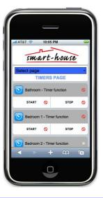
The hours, minutes and seconds can be changed touching the relative box: its background will become yellow, and with + and - the desired numbers can be selected.
