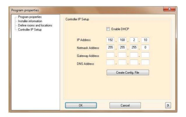
The DHCP addressing can not be used when the web server functionality is used because the assigned IP might not be always the same: you have always to configure a fix IP to connect to iSH web server. This means that if the "Enable DHCP" box is checked, you have to deselect it.
