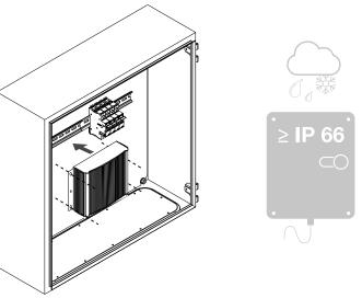
Note: For outdoor installation, a cabinet with an IP66 or higher protection degree must be used.
