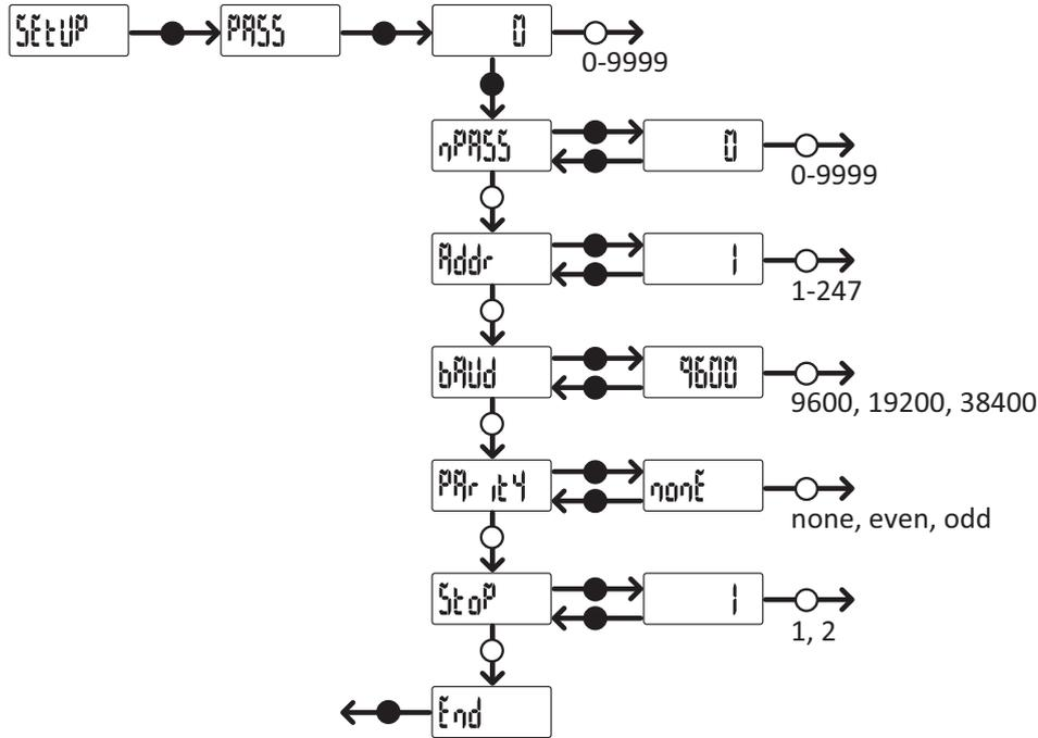
**Note:** to save the set value, press and hold down the button for about three seconds. To clear changes, wait 20 seconds.
