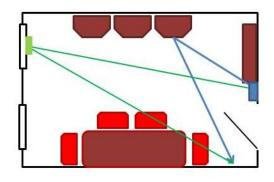
Attention has to be paid to metal panels, metallised glass windows or mirrors, which reflect the majority of the incident power, preventing the signal from passing through. However, some radio power may propagate through small apertures.
