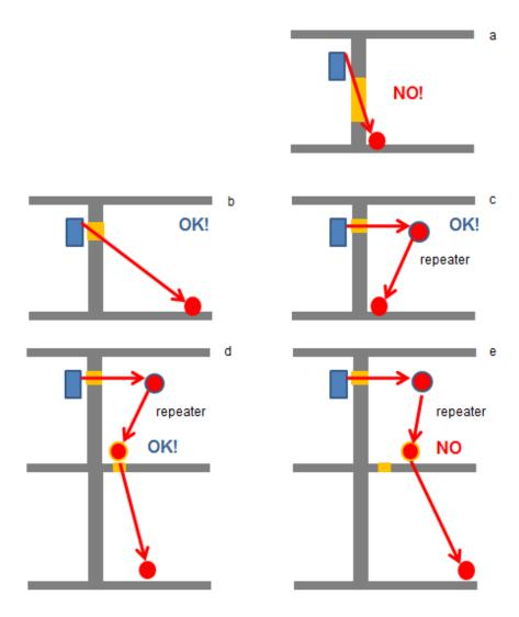
How to install the wireless modules in the smart Dupline system
