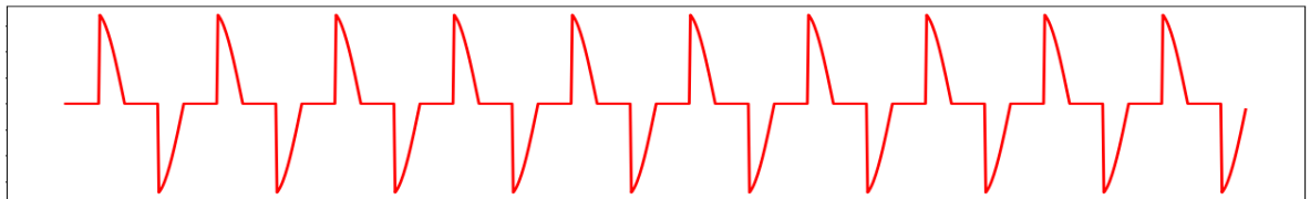
Output with Phase angle firing mode @ 33% control level
