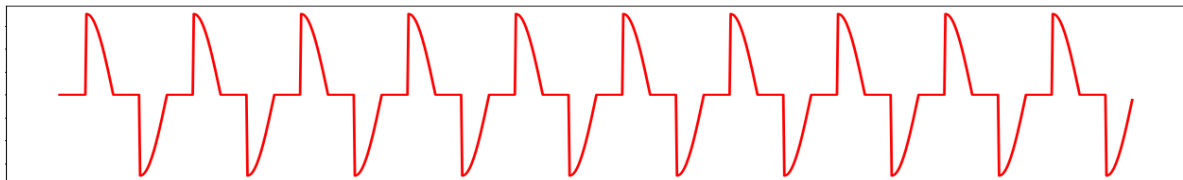
Output with Phase angle firing mode @ 50% control level
