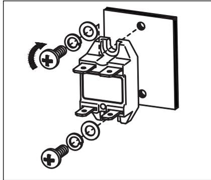
2. Tighten screws alternately to max. 1.0Nm.
