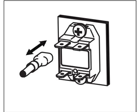
3. Insert / remove FASTON receptacle only with RF1 tightened to a surface.
