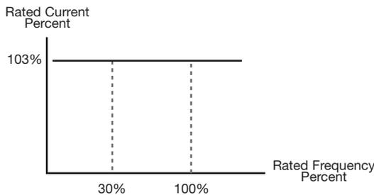
Inverter Duty Motor OL1 Protection Curve
