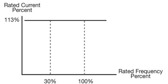
Inverter Duty Motor OL1 Protection Curve
