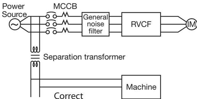
(A) Main circuit's wiring must separate from other high voltage or high current power line to avoid noise interference. Refer to the figures below:
