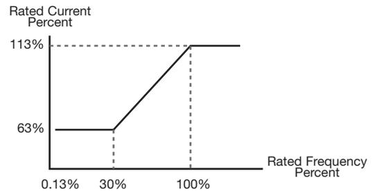
Non-Inverter Duty Motor OL1 Protection Curve
