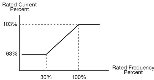
Non-Inverter Duty Motor OL1 Protection Curve
