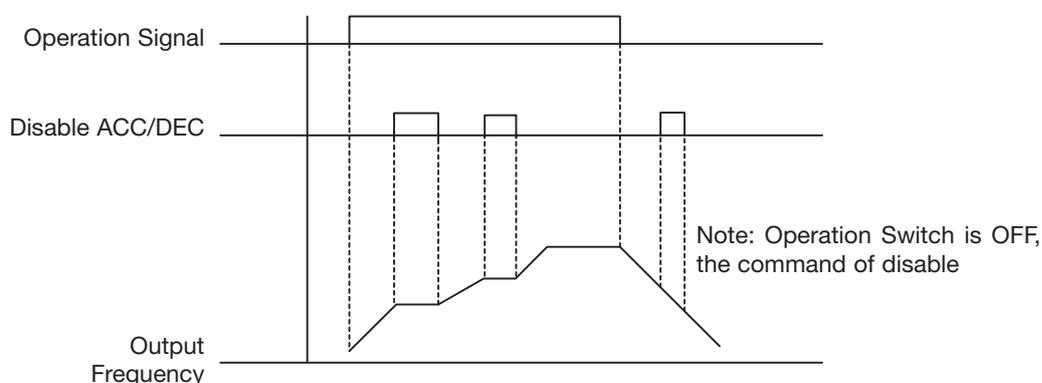
**L. 5-00~5-06=0014,0015: UP / DOWN Function (Actual ACC/DEC time is base on the setting):**
