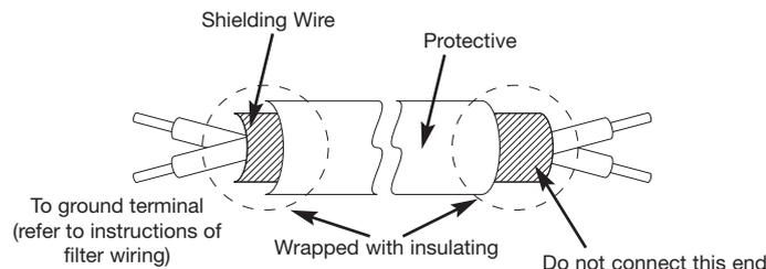
(C) Ground the ground terminal of the inverter properly. For 230V class ground 100Ω or less; for 480V class ground 10Ω or less.
