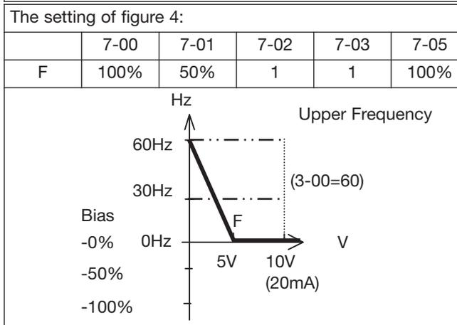
The inverter reads the average value of A/D signals once per (7-04x4ms). Users can determine scan intervals according to noise in the environment. Increase 7-04 in noisy environment, but the respond time will increase accordingly.
