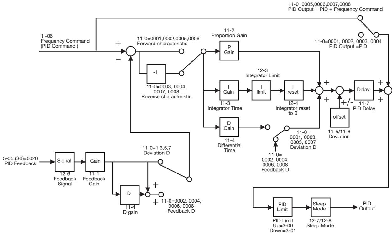
Performing PID control, set 5-05 or 5-12=0020, AI2 (S6) on TM2 as PID feedback signal. The target value of above diagram is the 1-06 input frequency. There are two ways to see the PID feedback signal, one is using the Keypad switch display (4-06 must be setting as 0001), the other is using analog output FM+ (8-00 must be setting as 0005).
