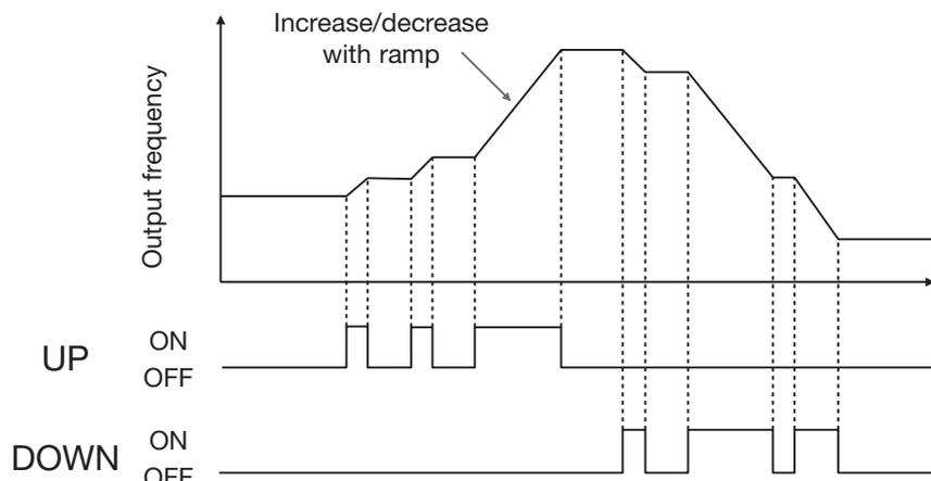
(2) 5-09 = 0.01 to 5.00, UP/ DOWN terminal ON, that equivalent to increase/decrease the frequency of 5-09. If the pressing is over 2 seconds, revive the original UP/DOWN mode (Please refer to the following diagram)
