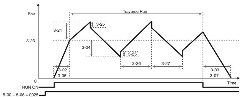
2) During traverse run, the center frequency could be controlled by the multifunction input terminals.
