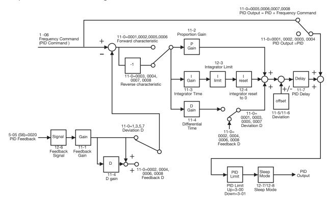
Performing PID control, set 5-05 or 5-12=0020, AI2 (S6) on TM2 as PID feedback signal. The target value of above diagram is the 1-06 input frequency.
