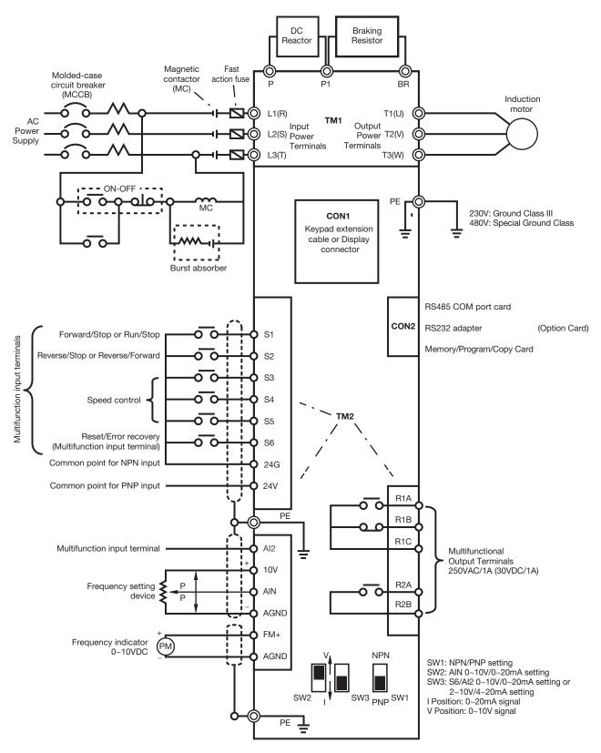
**Note 1:** Please refer to description of main circuit terminals (P1, BR) and specification of braking resistor for value selection.
