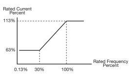
Non-Inverter Duty Motor OL1 Protection Curve OL=113% Start, 123%/1 Min.
