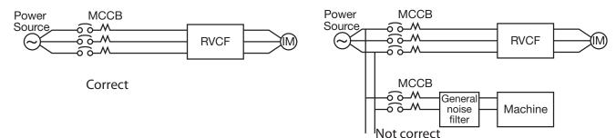
• Add a noise filter or separation transformer whenter shares the power line with other machines.
