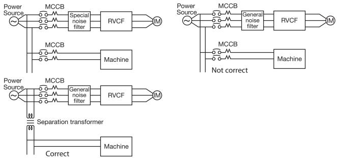
(A) Main circuit's wiring must separate from other high voltage or high current power line to avoid noise interference. Refer to the figures below:
