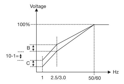
Note: 10-1=0.0, Torque boost function is invalid When the induction motor is in running, there must be slip due to the load. It is necessary to boost to improve the precision of the speed.
