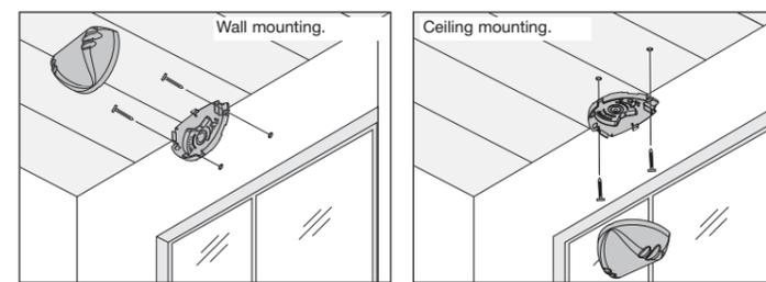
To install radar is necessary only a screwdriver and drill.
