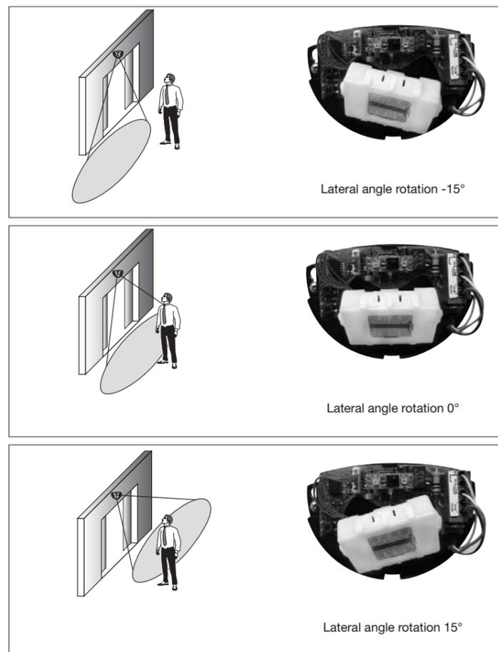
Adjust the lateral position to obtain the desired lateral angle sensing field.
