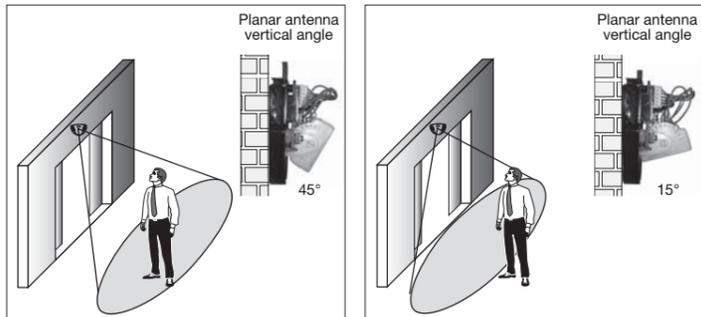
Adjust the vertical position to obtain the vertical sensing field close or far from the door.
