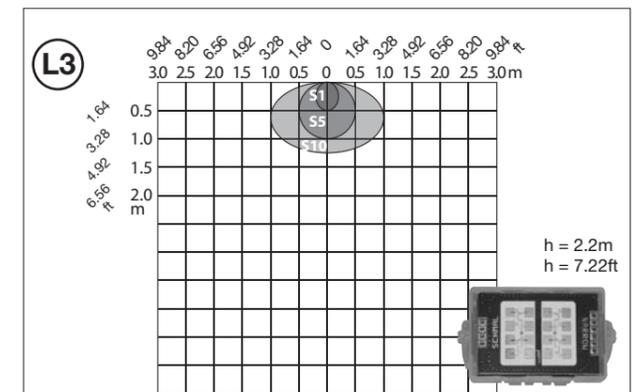
Detection area vs Sensitivity value (vertical angle 45°).
