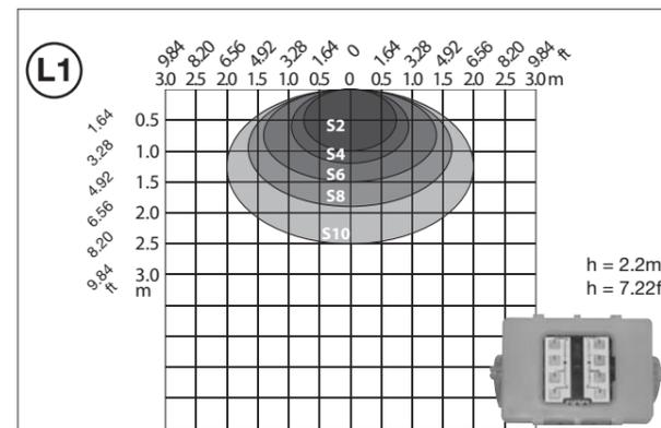
Detection area vs Sensitivity value (vertical angle 45°); horizontal mount mode.
