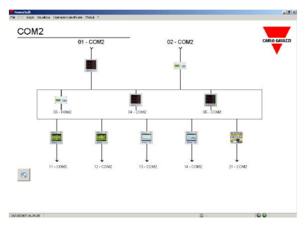
Any alarm status of each instrument is directly available on the synoptic pages: if the instrument is not communicating, a fuchsia square appears around it; if there is a setpoint alarm, the square indication is red.
