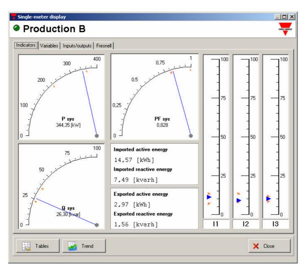
On the top of the page, the name of the instrument and the communication status are shown. The flashing of the green LED indicates that a new reading has been preformed from this meter and that the displayed values have been updated.
