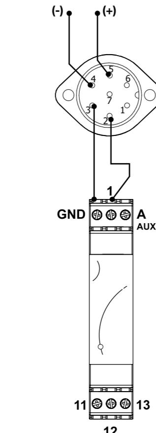
Note: the power supply unit MUST NOT be the same used for the Eos-Array which includes the VMU-P module.
