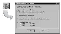
automatic configuration of the GSM modem. Follow the instructions given in the dialog box, then verify that the connections related to the communication between modem and PC are ok and finally click the "OK" button.
