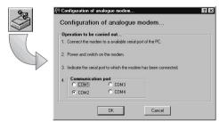
**Automatic configuration of analogue modem:** it allows the automatic configuration of the analogue modem. Follow the instructions given in the dialogue box, then verify that the connections related to the communication between modem and PC are ok and finally click the "OK" button.
