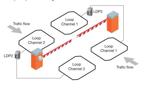
When the Automatic Channel Mode is selected, the Loop Detector scans all four channels during the first 10 seconds after start up. Based on this measurement the Loop Detector selects the channel which is least exposed to disturbance from neighbouring loops and other electrical or magnetic sources of noise. After automatic channel selection is completed, the power LED flashes white to indicate which channel is selected e.g. three flashes shows channel three is selected.
