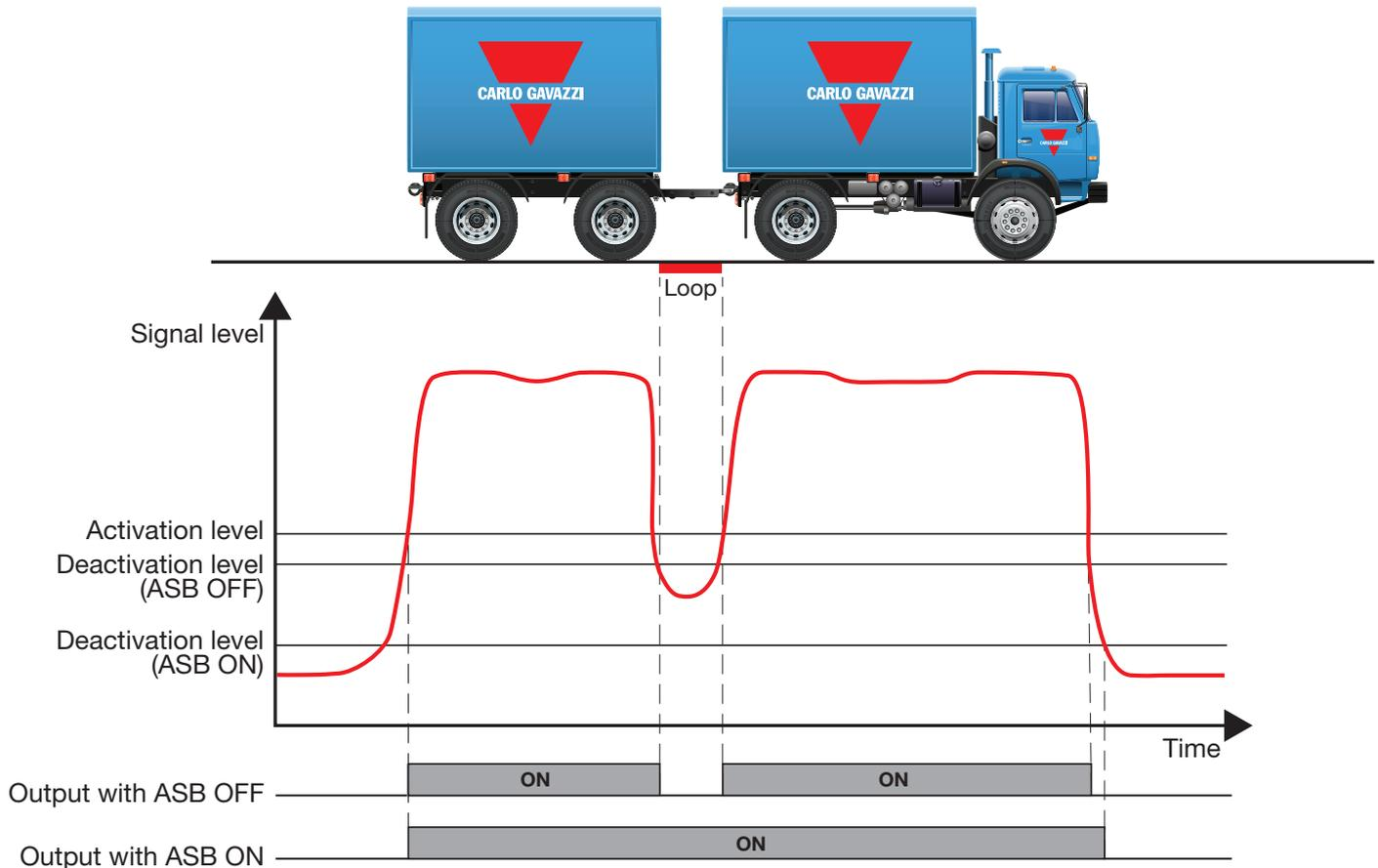
The sensitivity adjustment dial works in the same way with or without ASB function ON, by lowering or increasing the activation threshold. However by utilizing the ASB function it is possible to have correct detection of high bed vehicles for lower sensitivity settings.
