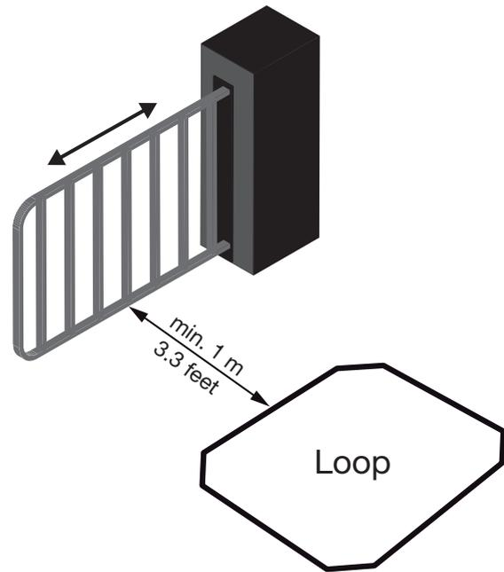
The length of the loop (b) influences the maximum speed at which a vehicle can be traveling and still be detected. For applications where detection of high speed vehicles is needed, it is important to consider this length. The table below shows relation between loop length (b) and maximum vehicle speed. The table below assumes correct adjustment of the Loop Detector sensitivity and a minimum vehicle length of 2.5 meters.
