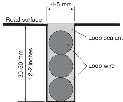
The recommended groove depth is 30-50 mm (1.2-2.0 inches). If the wires are installed deeper than 50 mm (2.0 inches), the detection signal for the Loop Detector is reduced and detection of high bed vehicles can be compromised.
