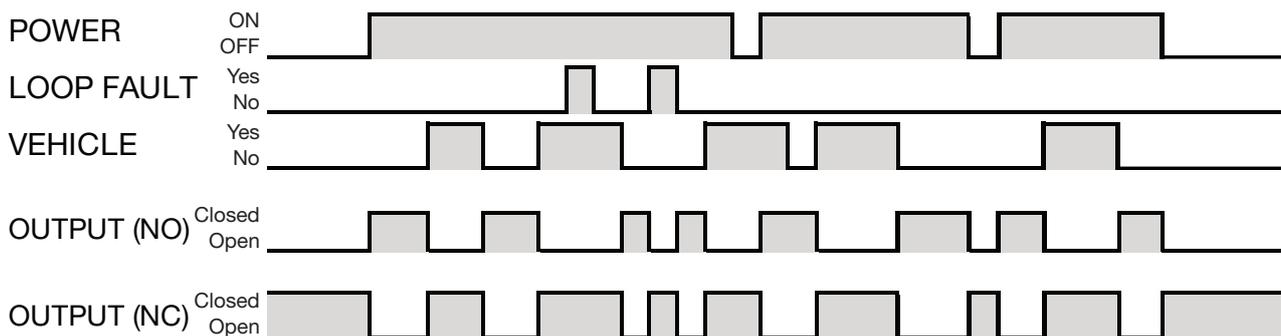
In Fail Secure mode the output relays operate normally while there are no issues in the application. If an error is detected or power to the Loop Detector is lost, the outputs will always fall back to default output state which is no vehicle detection in the loop. This function can be used if it is important to close the gate or barrier in case of problems.
