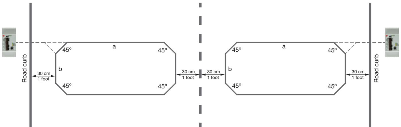
To reduce stress on the cable and thereby prolong its service life, it is important to avoid sharp bending of the cable. This is done by cutting a groove at 45 degree angles in each corner. The best signal condition for detecting a vehicle, is obtained when the width of the loop (a) is approximately the same as the track width of the vehicle. The width of the loop should therefore aim to have same dimension as the vehicles which needs to be detected.
