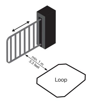
The length of the loop (b) influences the maximum speed at which a vehicle can be traveling and still be detected. For applications where detection of high speed vehicles is needed, it is important to consider this length. The table below shows relation between loop length (b) and maximum vehicle speed. The table below assumes correct adjustment of the Loop Detector sensitivity and a minimum vehicle length of 2.5 meters.
