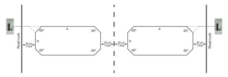
To reduce stress on the cable and thereby prolong its service life, it is important to avoid sharp bending of the cable. This is done by cutting a groove at 45 degree angles in each corner. The best signal condition for detecting a vehicle, is obtained when the width of the loop (a) is approximately the same as the track width of the vehicle. The width of the loop should therefore aim to have same dimension as the vehicles which needs to be detected.
