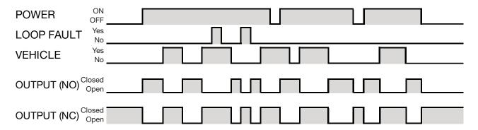
In Fail Secure mode the output relays operate normally while there are no issues in the application. If an error is detected or power to the Loop Detector is lost, the outputs will always fall back to default output state which is no vehicle detection in the loop. This function can be used if it is important to close the gate or barrier in case of problems.
