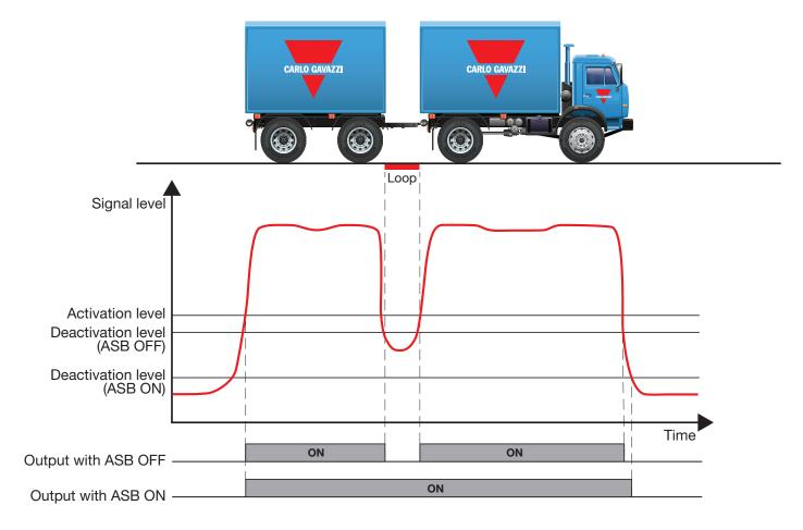
The sensitivity adjustment dial works in the same way with or without ASB function ON, by lowering or increasing the activation threshold. However by utilizing the ASB function it is possible to have correct detection of high bed vehicles for lower sensitivity settings.
