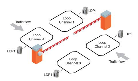
When the Automatic Channel Mode is selected, the Loop Detector scans all four channels during the first 10 seconds after start up. Based on this measurement the Loop Detector selects the channel which is least exposed to disturbance from neighbouring loops and other electrical or magnetic sources of noise. After automatic channel selection is completed, the power LED flashes white to indicate which channel is selected e.g. three flashes shows channel three is selected.
