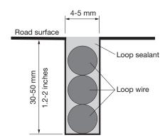
The recommended groove depth is 30-50 mm (1.2-2.0 inches). If the wires are installed deeper than 50 mm (2.0 inches), the detection signal for the Loop Detector is reduced and detection of high bed vehicles can be compromised.
