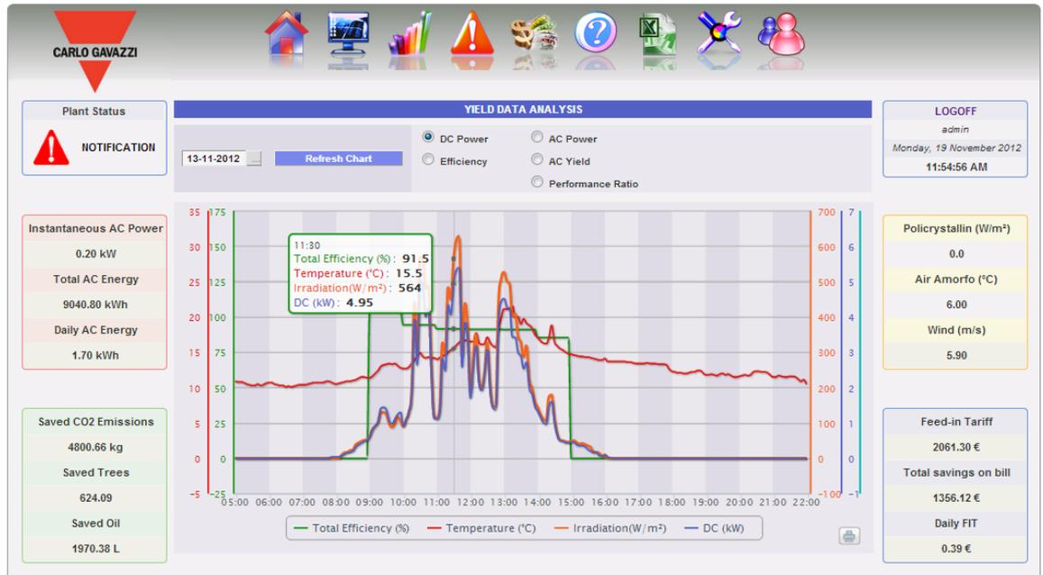
Fig. 101 - Production data analysis in DC chart
