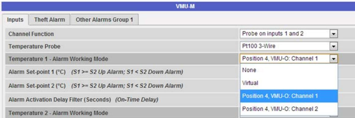
Fig. 65 – Mask for alarm configuration on VMU-M module
