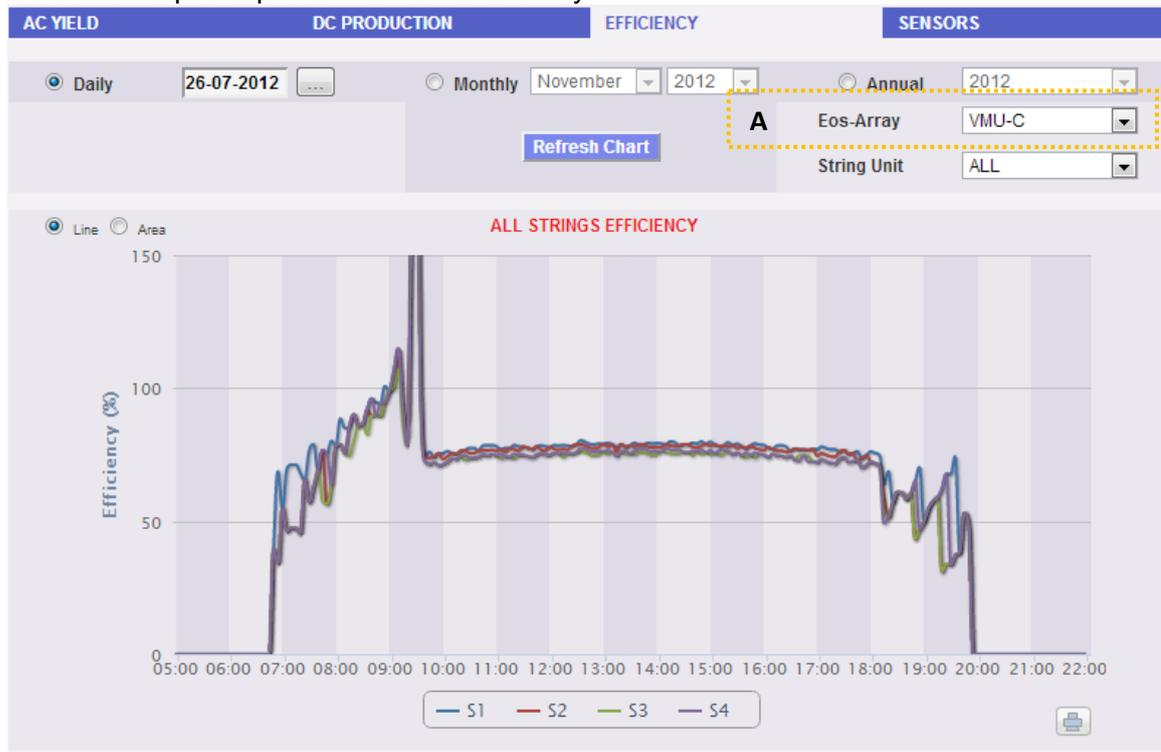
Fig. 132 - Single String efficiency
