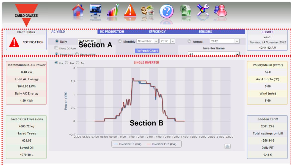
Fig. 115 - AC PRODUCTION - SINGLE INVERTERS chart
