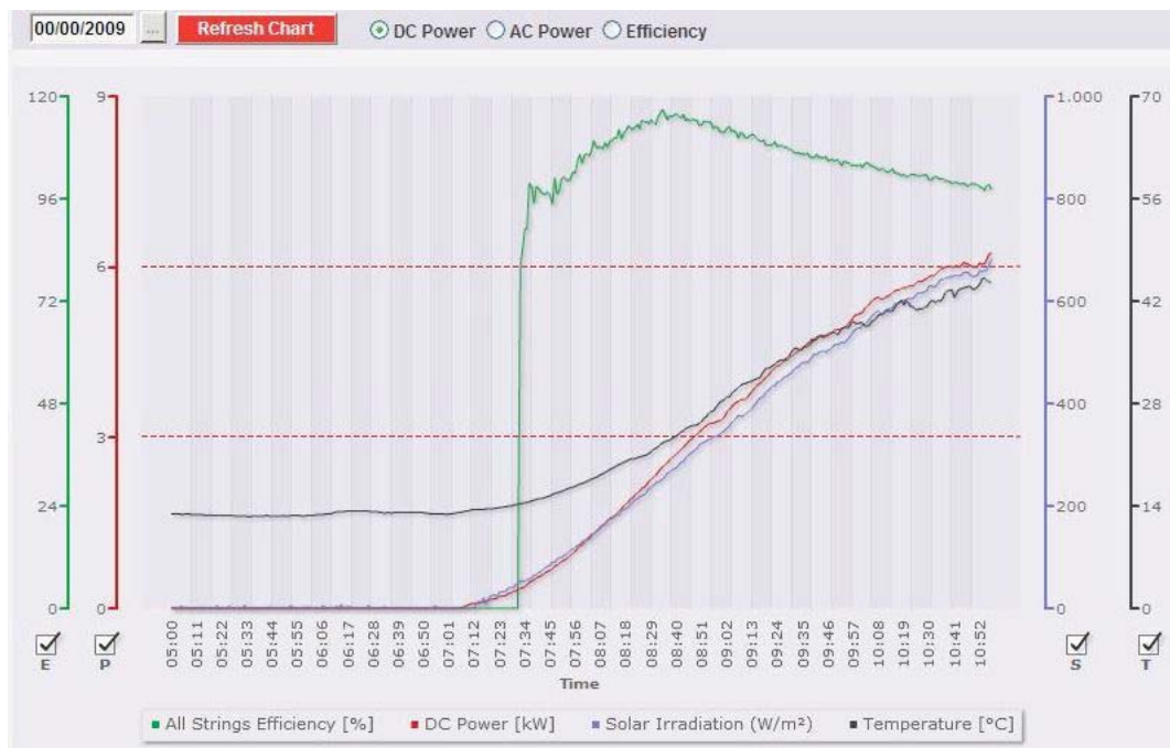
Fig. 70 - Production data analysis in DC chart
