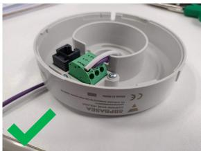
Leave some spare cable for each sensor (2/3 cm) in order to have enough cable to make the connection with the sensors connectors easier.
