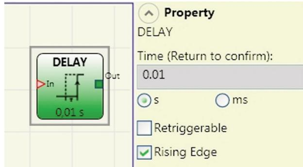
**Rising edge:** If selected, the delay starts on the input signal's rising edge at the end of which the output changes to 1 (TRUE) if the input is 1 (TRUE) where it remains for as long as the input stays at 1 (TRUE).
