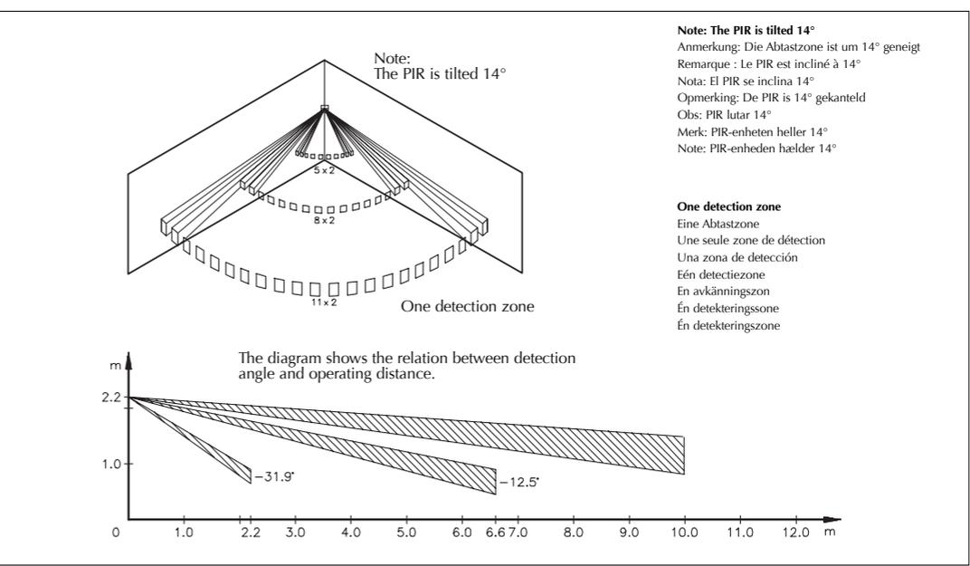
**The diagram shows the relation between detection angle and operating distance.**
