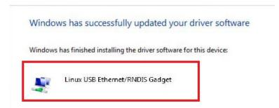
When the driver is installed, in the *Network adapter* category a virtual network board named *Linux USB Ethernet/RNDIS Gadget* will be added, as shown in the picture below:
