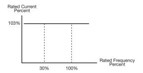
Inverter Duty Motor OL1 Protection Curve OL=103% Start, 150%/1 Min.
