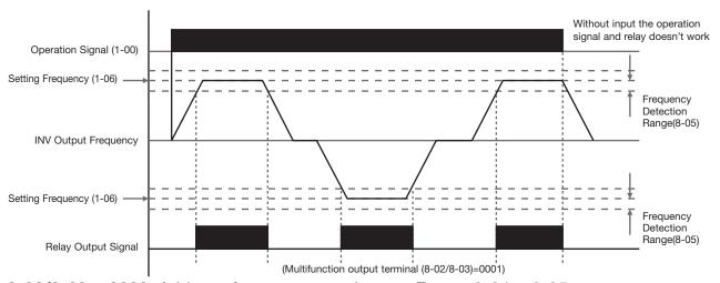
**8-02/8-03 = 0002:** Arbitrary frequency consistency Fout =  $8-04 \pm 8-05$  Operation Frequency Reached Arbitrary Frequency ( $8-04\pm 8-05$ ) Operation conditions:
