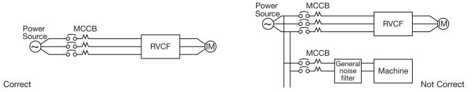
Add a noise filter or separation transformer whenter shares the power line with other machines.
