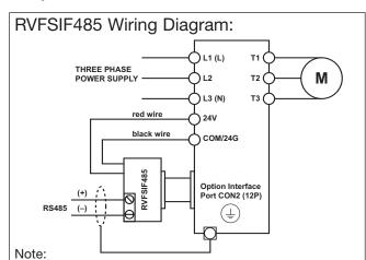
Please put on the cover of inverter to avoid the Interface Card disturbed by outside static electricity.
