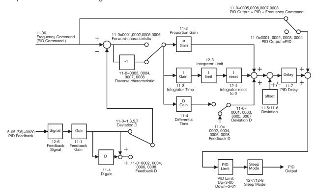
Performing PID control, set 5-05 or 5-12=0020, Al2 (S6) on TM2 as PID feedback signal. The target value of above diagram is the 1-06 input frequency.
