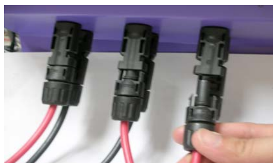
Fig 3.3.2.3 PV+ terminal connection
