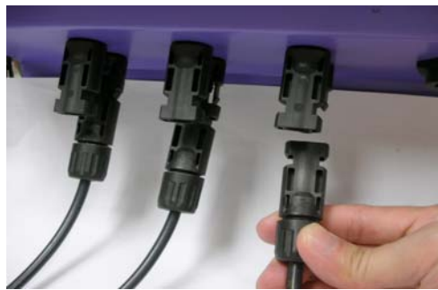
Fig 3.3.2.2 PV- terminal connection
