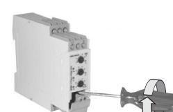
**⚠ Do not open the DIP-switches cover if the Power Supply is ON**
